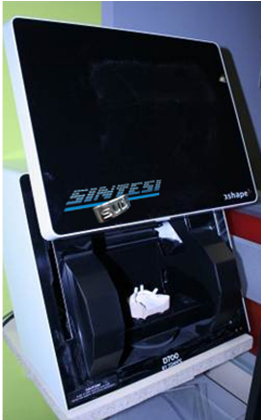
Fig. 6 – Shape acquisition of the pre-surgical cast with implant analogs.
